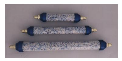
Trigon moisture traps utilize polycarbonate bodies, more inert and resistant to infusion than the acrylic used by other manufacturers. These traps are refillable and available in three sizes with three different adsorbent combinations. The ends are provided with Swagelok™ tube fittings. Each end fitting includes a 40 micron sintered stainless steel frit. Maximum pressure is 125 psi.
